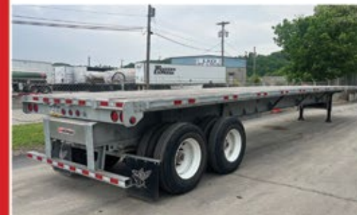
2017-2022 Manac Extendable Flatbeds (Galvanized & Painted), 48'102"-80' & 53'x102"-90' (Tandems and Tri Axles).
